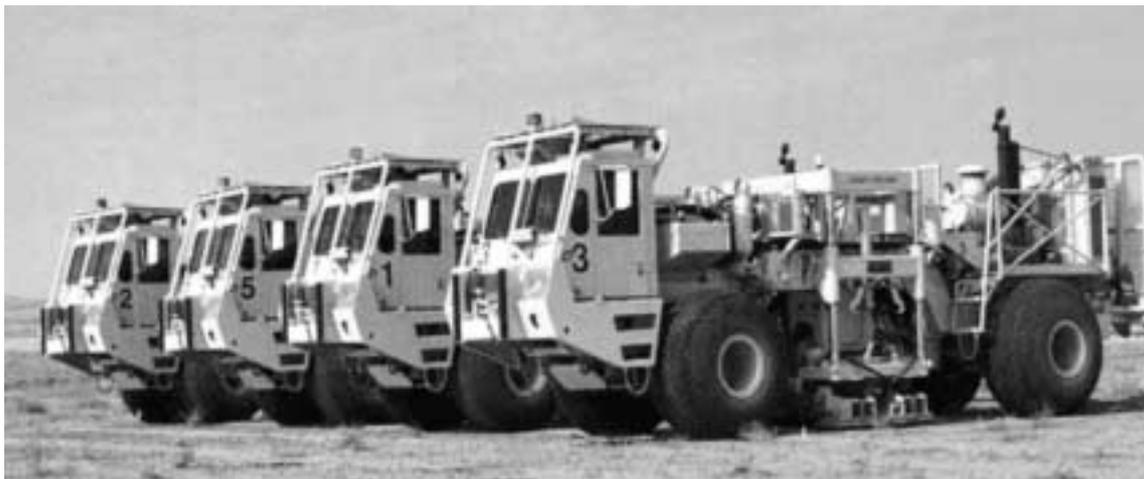
VibroSeis trucks used in recording seismic surveys onshore
